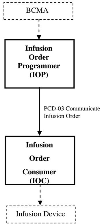
**Figure 4.1-1: Point-of-Care Infusion Verification Actor Diagram**
